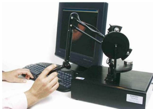
Fühlgriffel Geomagic PHANTOM Premium 1.5 HF 6DOF haptic device
